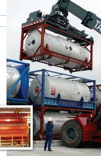
An NECDF employee helps guide a stacker operator as he safely maneuvers an intermodal container filled with hydrolysate. The intermodal containers are safely stored in the intermodal container storage area.
